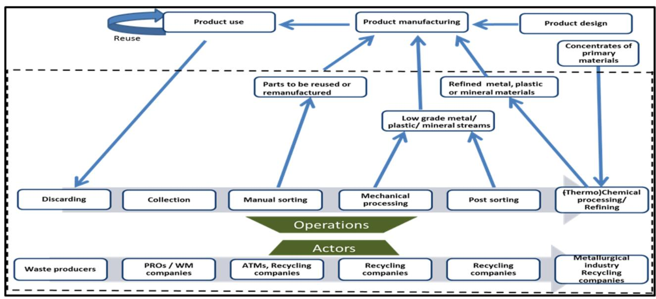
Figure 4: Process chain of ELV waste, excluding material loss due to incineration and landfill
